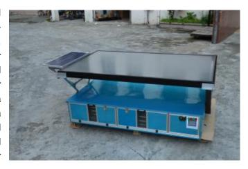
Model (shown on work table) with solar air collector set at 30 degrees. This setting is suitablefor temperate latitudes. The setting of the collector can be easily adjusted between 20° and 45° for the seasonal changes of solar angle or for various latitudes.
