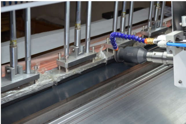
Aluminium absorber strip welding with copper tube
